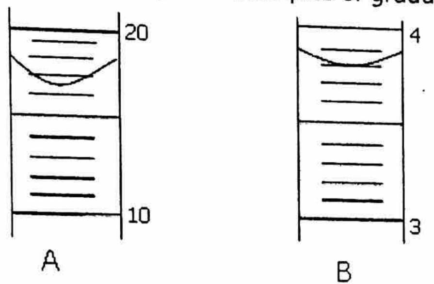
An important part of Chemistry is measurement. It is very important that you read the measuring devices we use in lab as accurately as possible. Here is how to determine how accurately a measuring device can be read:
