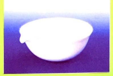
Evaporating dishes are used to evaporate excess solvents most commonly water to produce a concentrated solution or a solid precipitate of the dissolved substances.
